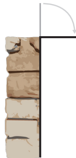
Bending the Flashing
